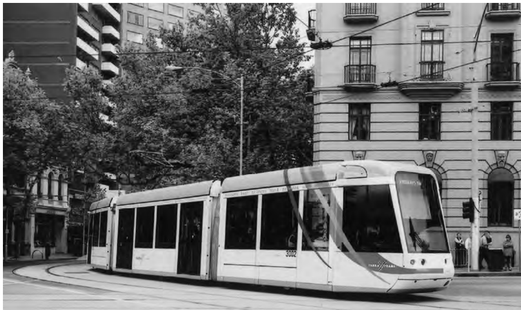
A new low-floor tram, the Citadis tram, operated by Yarra Trams.
