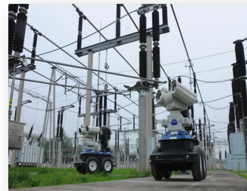
Substation Inspection Robots
