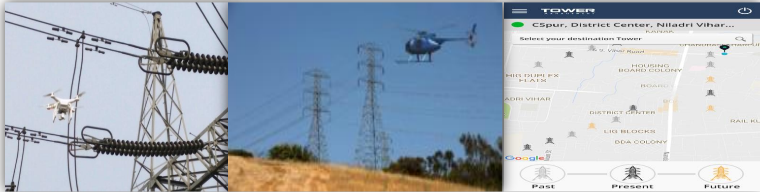
Patrolling of Lines through Drones, Helicopters and Tablet App based
