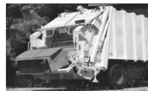
Mechanised bin tipping
