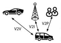
Cooperative Intelligent Transport Systems (C-ITS) are emerging technologies that allow road users and roadside infrastructure to share information with each other. Connectivity can be primarily between vehicles (V2V) or between vehicles and infrastructure (see Vehicle to Infrastructure (V2I) Connectivity and Smart Motorways use case).
